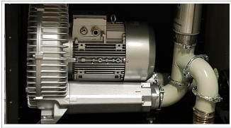
The blower is placed in a sound absorbing box. An additional duct silencer on the outlet of the unit further reduces the sound level.
