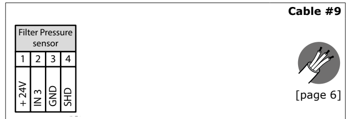
Fig. 4.20 Connection of external pressure sensor
