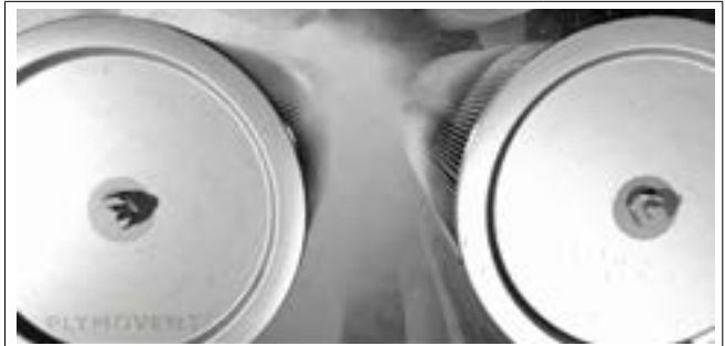
The effective RamAir™ pulse amplifier: individually cleaning of the filter cartridges by compressed air pulses
