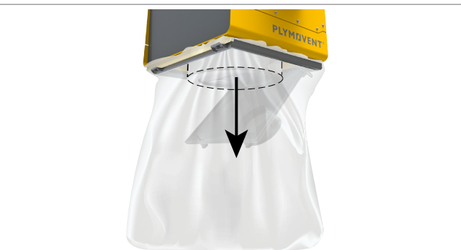
Dammfritt filterbyte & service (bag-in/bag-out)
