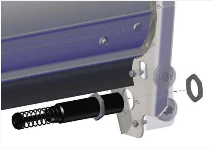
Fig. 5.3.5 Mounting the hydraulic shock on the cover plate
