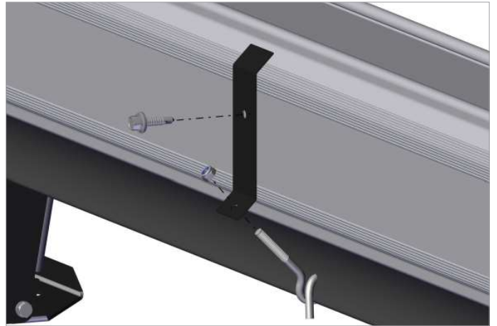
Fig. 4.3.9 Mounting the rope bracket
