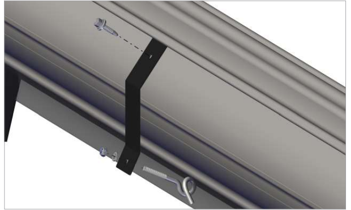
Fig. 5.3.8 Mounting the rope bracket
