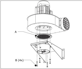
Fig. 4.4 Fan on arm bracket
